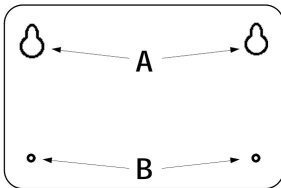
**NOTE:** You may install the timer using two screws aligned horizontally.
