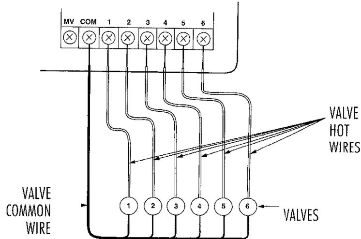
Connect the one common wire (usually the white strand) to the terminal labeled "COM". Connect the second "hot" wire (usually the color-coded strand) from each valve to one of the terminals numbered 1 -6 on the number of stations on your timer model. Connect wire from valve 1 to terminal 1, valve 2 to terminal 2, etc.
